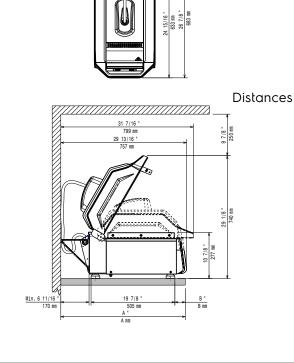
Plug In SpeeDelight with flexible top plate, ribbed, removable teflon plate
